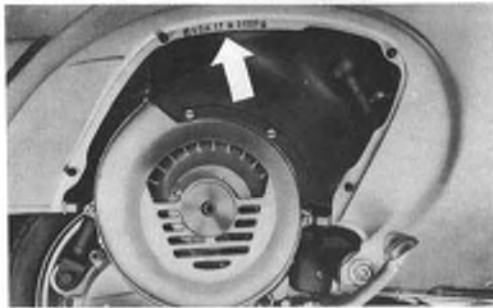
Fig. 24 - Serial number stamped on frame. scooterhelp.com
