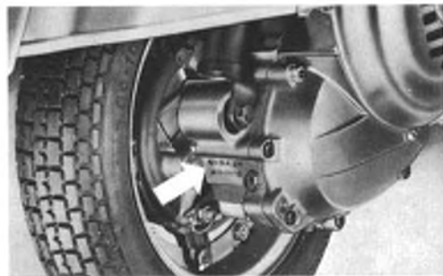
Fig. 23 - Serial number stamped on engine.
