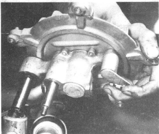
3.9a Detach hub as a complete unit
