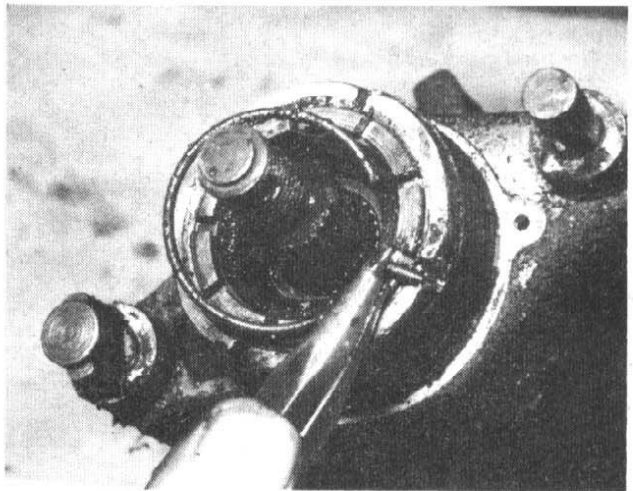
5.3 Bearing retainer has an oil seal within the centre
