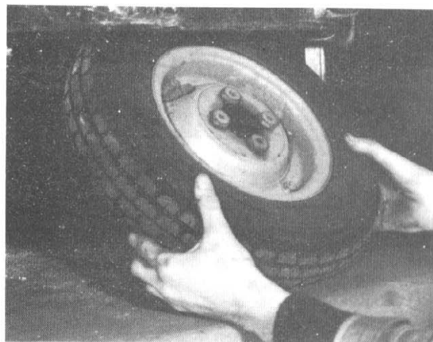
5.3b Wheel will pull off splined shaft
