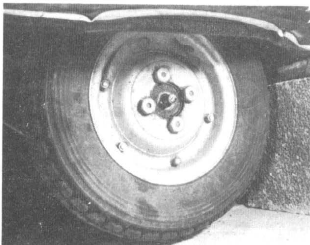
36.5a Rear wheel will slide onto splined shaft
