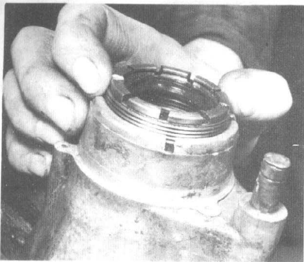
29.1b Tighten bearing retainer fully
