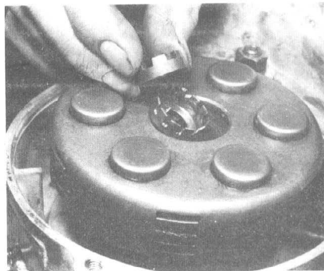
30.1c Fit tab washer and tighten centre nut with peg spanner
