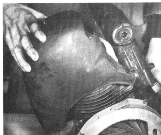
8.1 Engine cowl is retained by a single bolt
