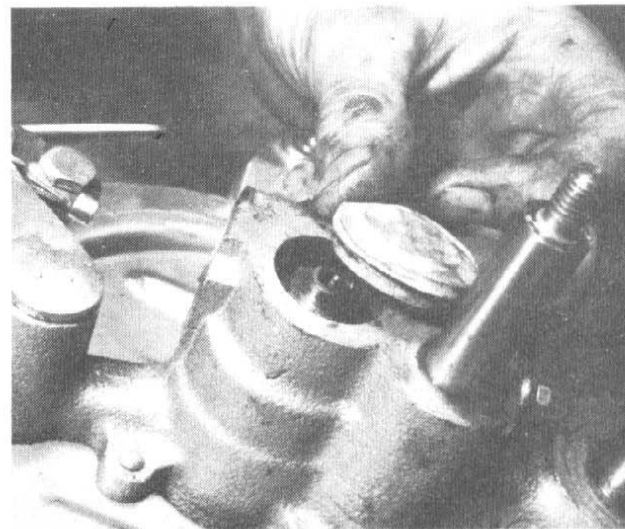
3.11a Rubber plug blanks off end of stub axle
