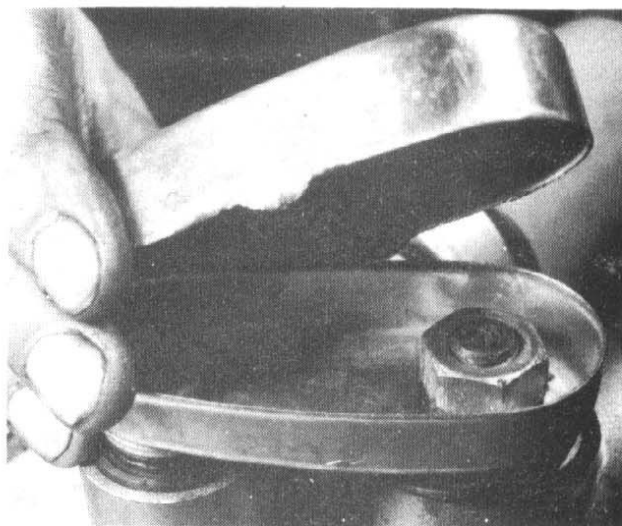
3.8b Prise back lugs to remove cover
