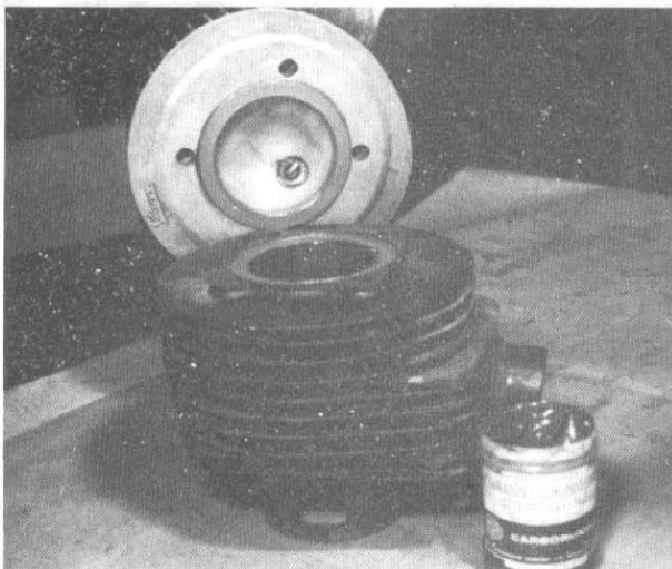
20.5 Use valve grinding compound to lap-in cylinder head joint
