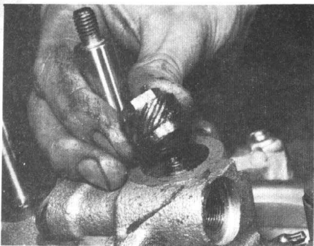
3.11b Speedometer drive pinion nut has left-hand thread
