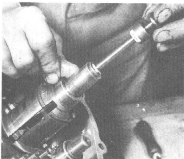
13.3b Lift out rod and rod holder ...
