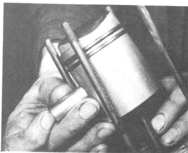
32.2 Gudgeon pin should press into position
