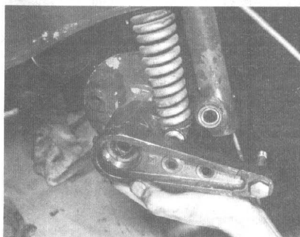
3.6d Stub axle housing can be lifted away for bearing attention
