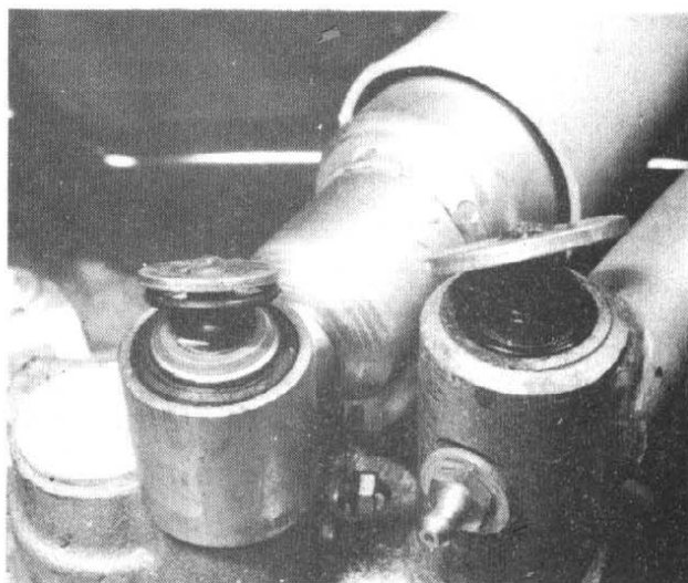
3.8d ... 'O' ring seals are under washers
