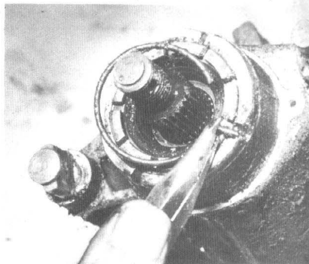
13.4a Wire clip locks bearing retainer
