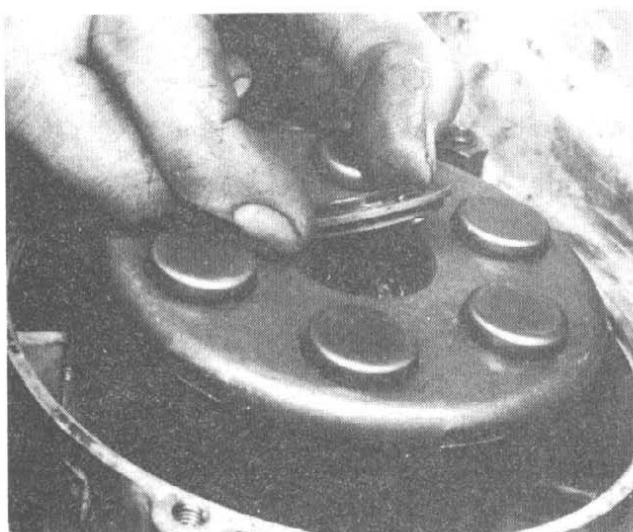
30.2 Replace thrust plate in centre
