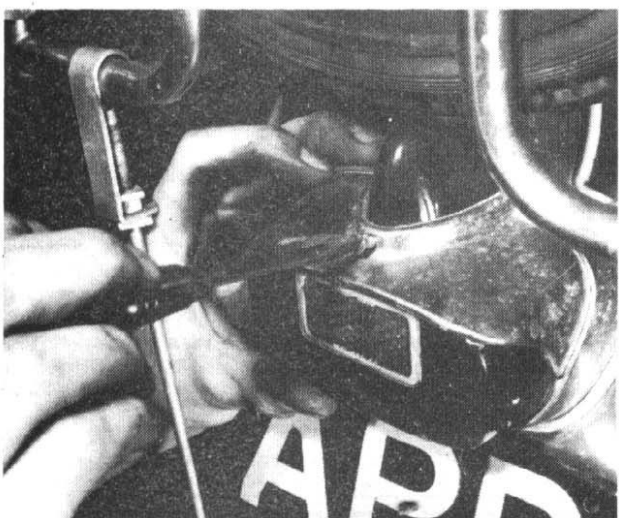
9.1 Single screw retains rear lamp cover
