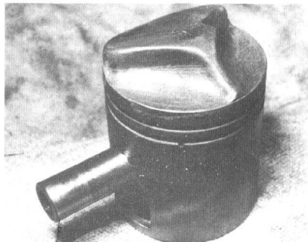
11.3c Mark piston inside skirt to ensure replacement in correct position
