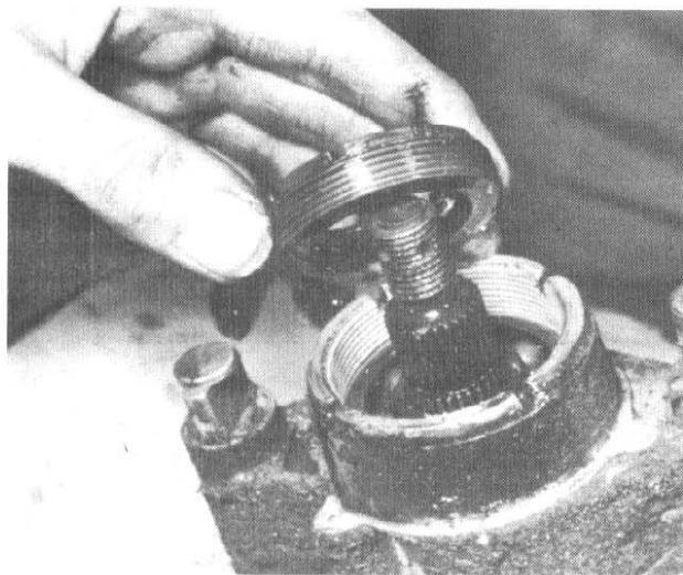
13.4b Unscrew bearing retainer for access to bearing
