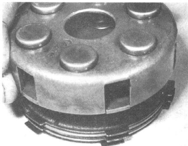
25.6 Reassemble, pressure plate uppermost
